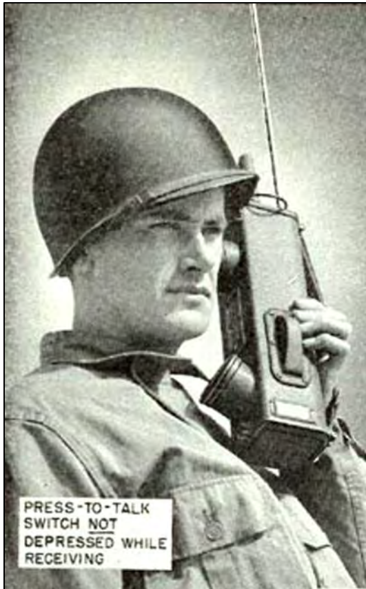
Walkie-Talkie, Model SCR-536. With a range of two or three hundred feet, this Walkie-Talkie weight about 5-pounds and was found at company level. Image source: War Department Technical Manual TM11-235.
